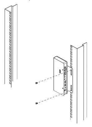
**Note:** These screws are not provided. We recommend that you use M5 x 12 Phillips Type I cross, recessed type screws.
