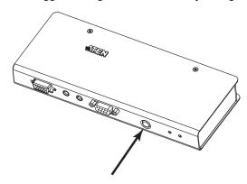
**Note:** Remote mode cannot be selected. The remote console can get control only when the Operating Mode Pushbutton on the CE750L is toggled to *Auto* and the local console is idle. If the remote console is then idle for more than five seconds, the local console can gain access.
