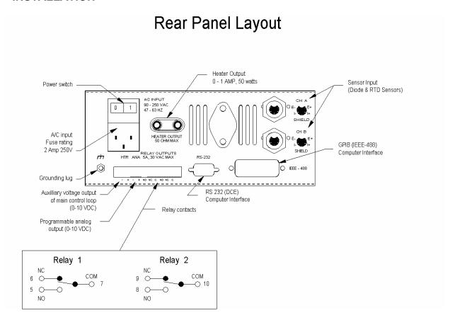
Hardware installation consists of making the proper connections between external devices and the rear panel shown above. The minimum connections are as follows:
