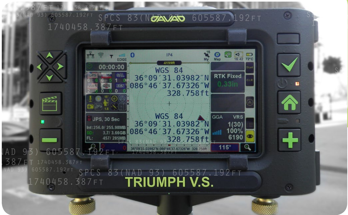
Even in a high multipath environment, the V.S. quickly fixes and provides a very good precision solution.
