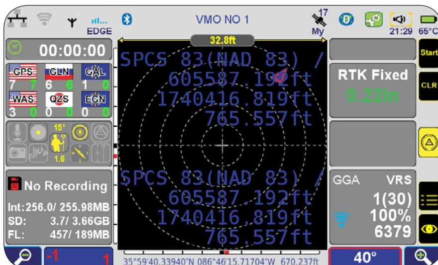
The "Action" Screen provides extensive status and positioning information in one view.
