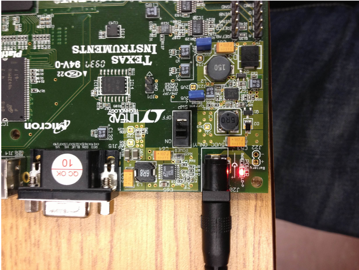
Image 4: Proper power connection
