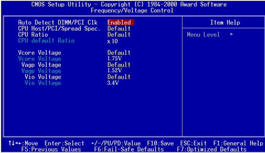
**Auto Detect DIMM/PCI Clk:** When enabled the motherboard will automatically disable the clock source for a DIMM socket which does not have a module in it. Same applies for PCI slots. This setting will reduce the EMI. The default is Enabled.
