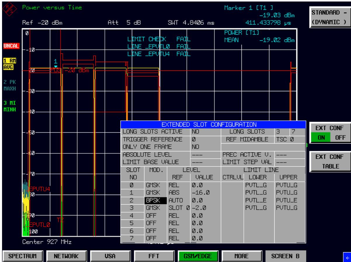
Fig. 2-10 Dynamic extended slot configuration
