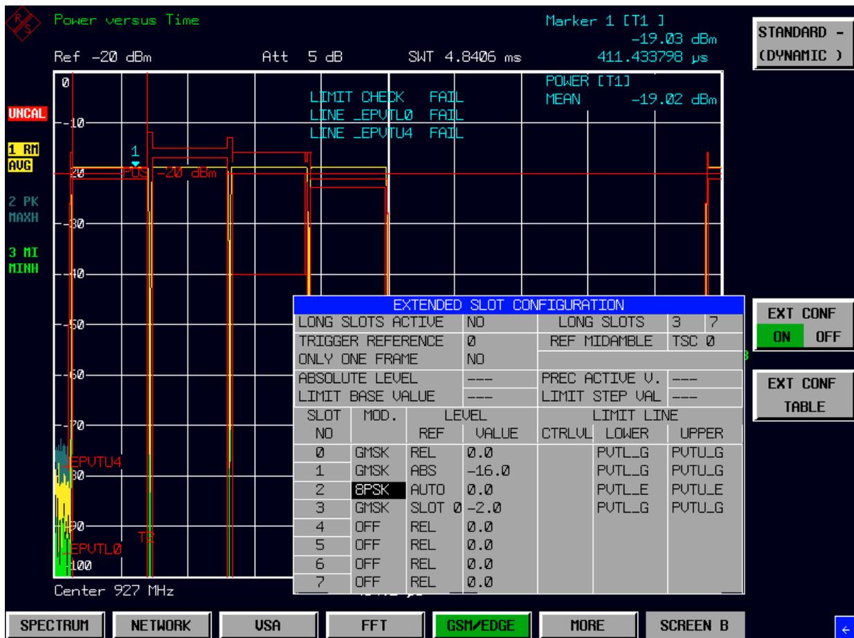
Fig. 2-9 Dynamic extended slot configuration – incorrect level
