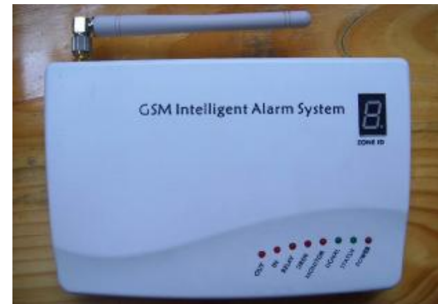
Figure1. the main panel of the alarm system
