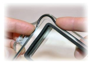
• The O-ring can be extracted using an O-ring extractor tool (make sure the tool as no sharp edges). Alternatively use the flats of the thumbs to gently stretch the O-ring on two faces thus making a small loop protruding a few mm. The loop can then be grasped between finger and thumb, to pull the O-ring over the lip.
