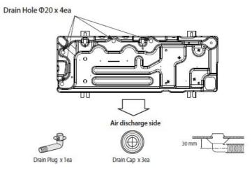
is used it must be 25mm longer and wider than the base of the unit to catch all the drips.
