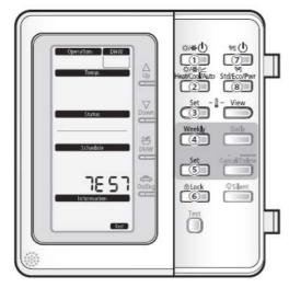
Press the **top left** button the unit will run the pump.
