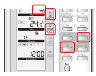
symbol shows at the top of the screen with 2 dots press set, adjust hours with up or down button to 3 am press set, minutes flash press set. Now everything flashes press set (grey). No 2 appears do the same again but for 15-00.
