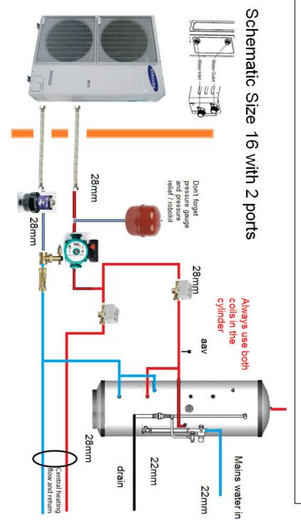
The 16 kW unit has 1 inch BSP male connections, these should be connected to flexi hoses (supplied).
