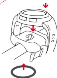
Assemble the handlebar holder.
