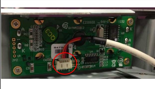
**Fig.2-14** Remove the EZIO cable from EZIO
