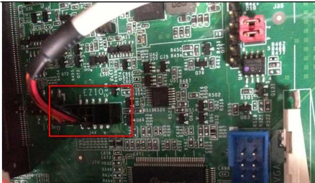
**Fig.2-16** Remove the front panel cable from main board
