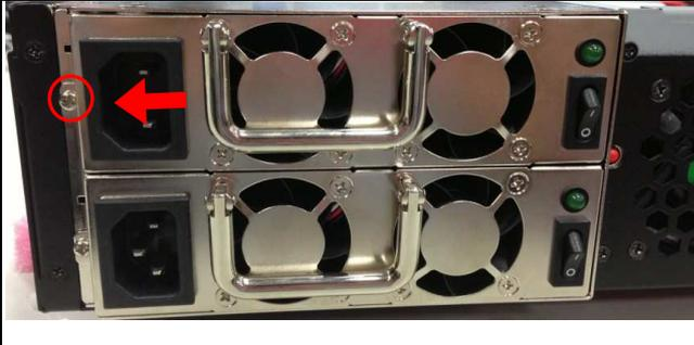
**Fig.2-21.1** Remove the screw to unlock the power module.
