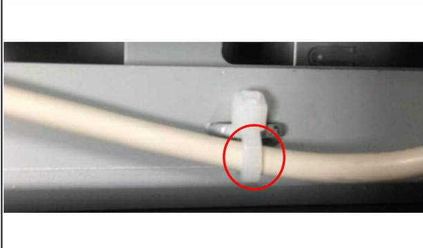
**Fig.2-15** Cut the cable collector.
