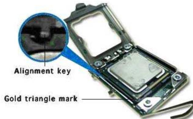
6. Close the load plate (A), then push the load lever (B) until it snaps into the retention tab
