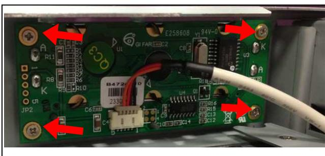
**Fig.2-18** Remove the screws from EZIO kit
