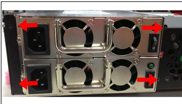
**Fig.2-25.1** Remove the screws.
