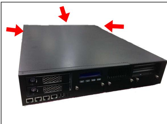
**Fig.2-17a** Please loosen the screw of top cover: two at the left and right side, last one at the rear side, to remove the top lead
