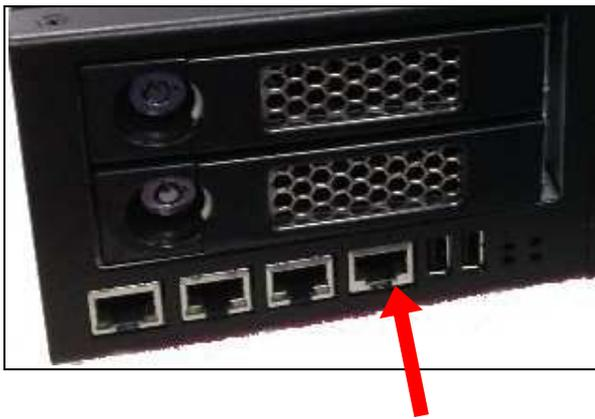
**Fig.2-36** Connect null serial port cable to CAR-5030 console management port.
