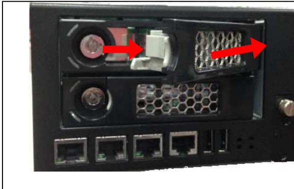
**Fig. 2-12a** Connect HDD bracket to CAR-5030 system then push the switch in.
