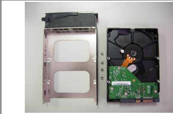
**Fig. 2-11a** A 3.5" SATA HDD and the HDD bracket
