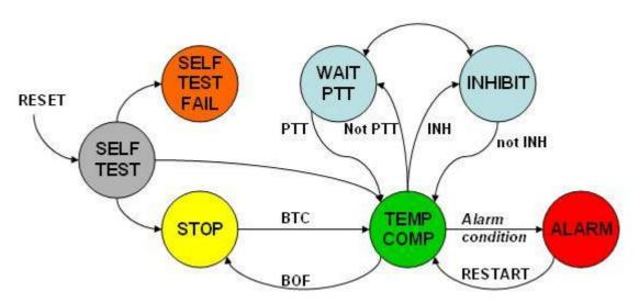
When switched on it runs an initial self-test, which lasts about 20S and that evaluates if the hardware is working correctly, running a series of checks:
