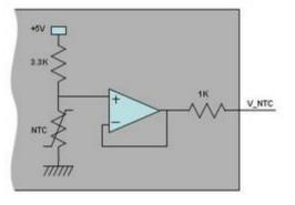
The NTC is internally powered at 5V through a 3. 3 kOhm resistor and voltage is put out through an analog buffer. From the voltage value, through an appropriate processing, it is possible to trace the value of resistance R(T) of the NTC
