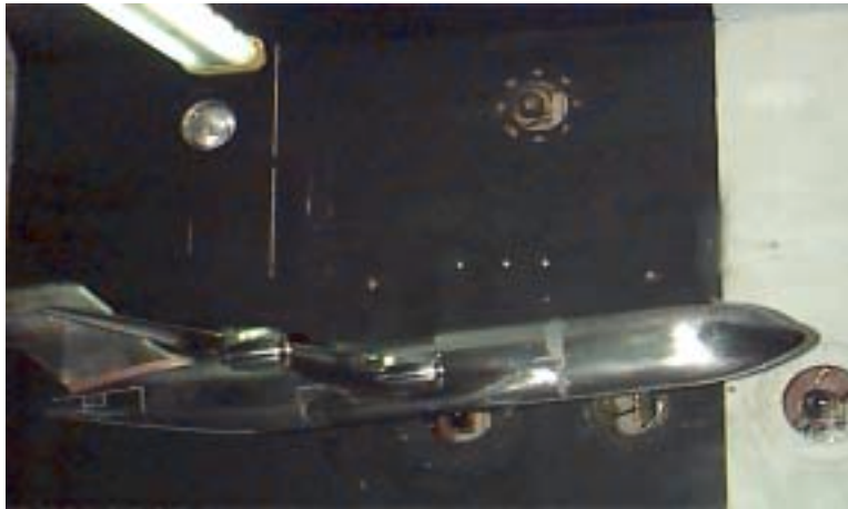
Figure 11. Tunnel wall painted flat black for contrast.
