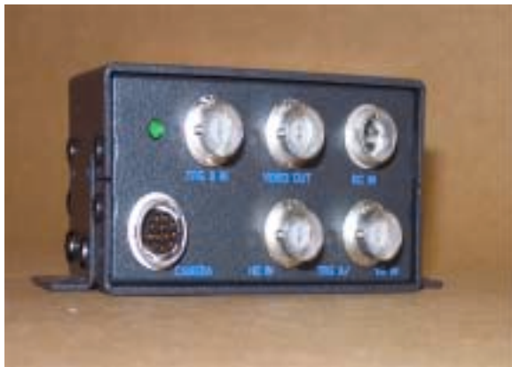
Figure 3. Cable Junction Box for Hitachi Camera.
