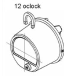
Do not remove the magnet from the meter's reed switch while communicating through the meter's IR port.
