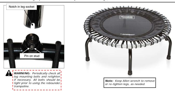
**2)** With trampoline upside-down, fit leg sockets over stud on trampoline frame. Notch in leg socket lines up with pin on stud. All leg hardware fits inside of each leg socket, in the order shown in Step 1. Securely tighten Allen bolts with supplied 6mm Allen wrench. If you are going to install an exercise handle, turn to next page for installation. When all legs are installed, turn your rebounder over.
