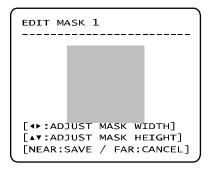
Adjust mask size. Use joystick or arrow buttons to adjust mask size.
