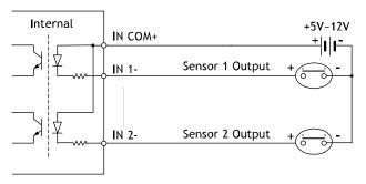
Before connecting sensors, check driving voltage and output signal type of the sensor. Since output signal types of the sensors are divided into Open Collector and Voltage Output type in general, the cabling must be done properly after considering these typed.
