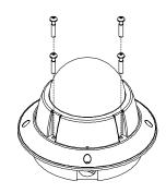
③ Wire cables to terminal block and connect the terminal blocks to main unit. Screw main unit to surface mount bracket with 4 lock-up screws.
