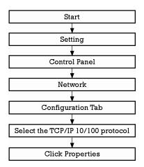
• Note the settings under the IP Address, DNS Configuration, and Gateway tabs
