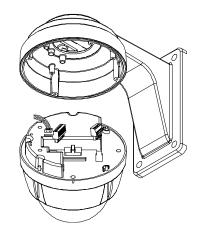
3 Screw main unit to wall mount bracket with 4 4 Detach protection vinyl from dome cove. screws.
