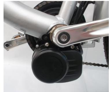
The nominal speed is 90 revolutions per minute, the nominal performance is 250 Watt and the maximal performance is 400 Watt.
