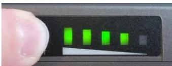
The state of charge of the battery you can control on the integrated display on the battery, when you push the red button. The battery is empty if only the red lamp is light.
