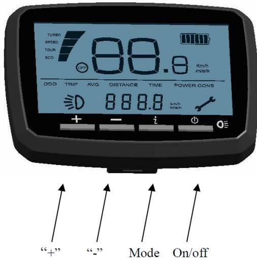
⏻ Press this button to power on the LCD display, Long pressing the button for 2 seconds to power off. Automatically shut off without any operation in 5 minutes.
