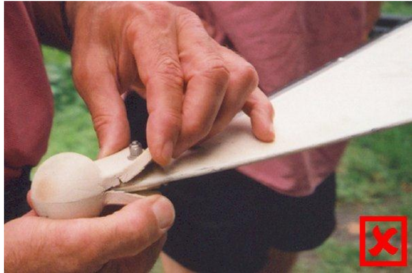
Bow Ball cracked and perished – Not Acceptable
