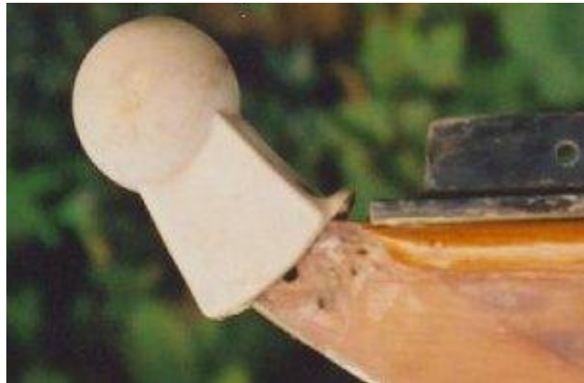
Bow Ball not secured – Not Acceptable
