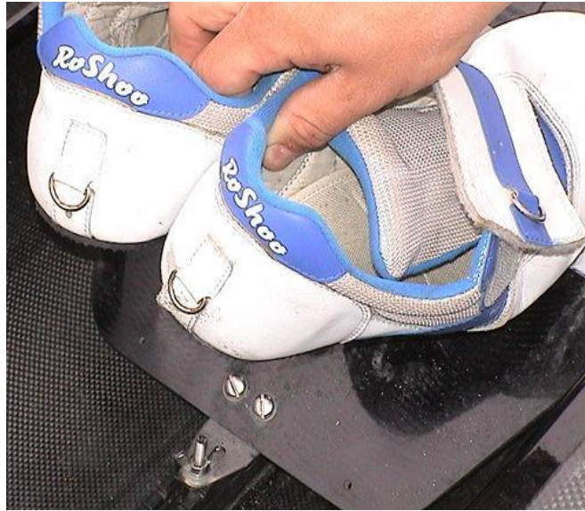
No Heel restraint strings tied– Not Acceptable
