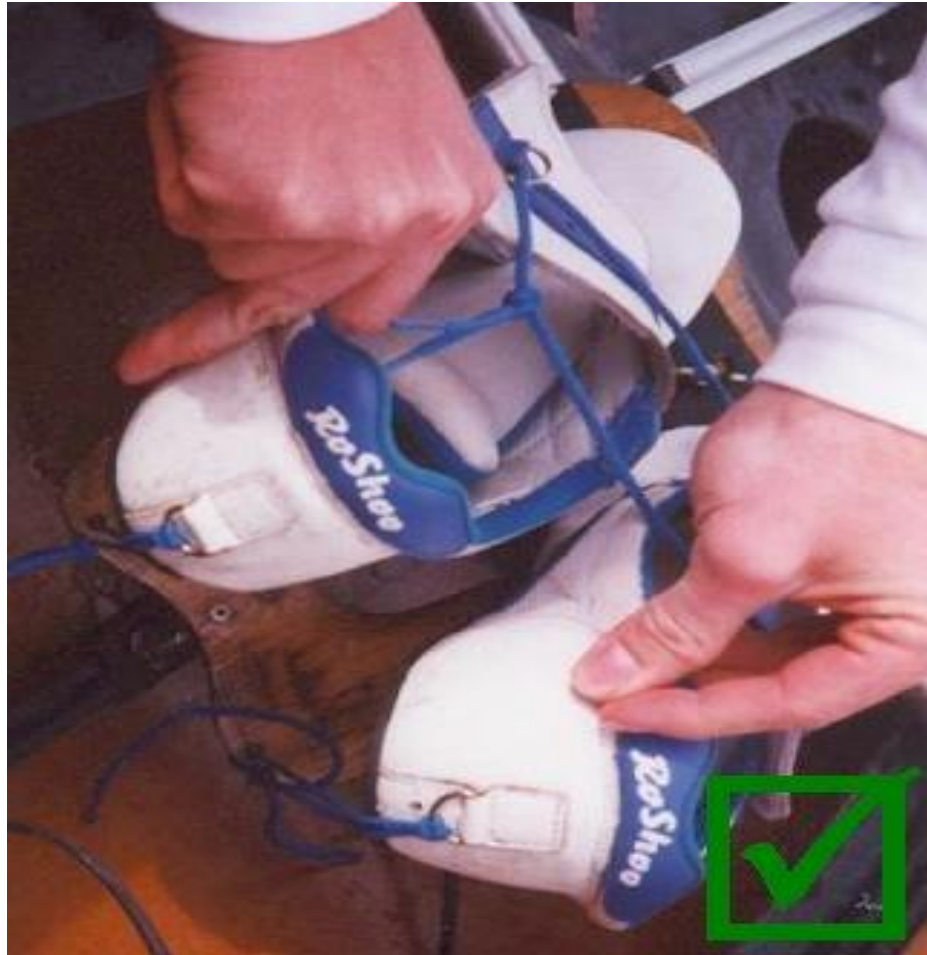
Heel restraints properly tied in - Acceptable
