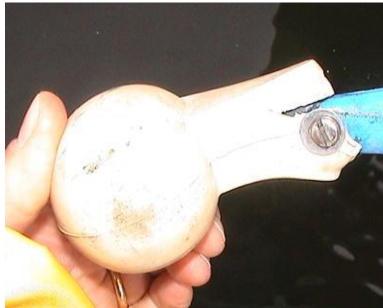
Bow Ball starting to crack – Not Acceptable
