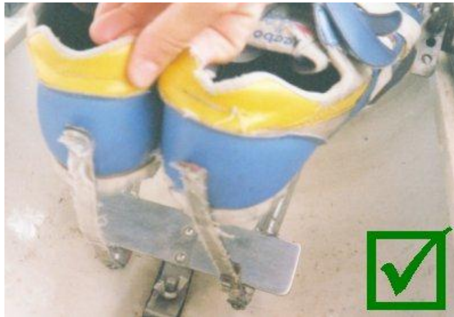
Heel restraints properly and individually secured – Acceptable
