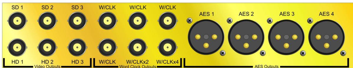
**HD Tri level sync** outputs, 3x 75 ohms BNC individually buffered & fully DC Coupled 1v video.
