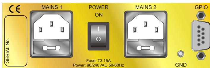
Fused mains input and common mains switch. Voltage input can be between 100v to 250v 50/60Hz and is mains filtered to enhance EMC performance.
