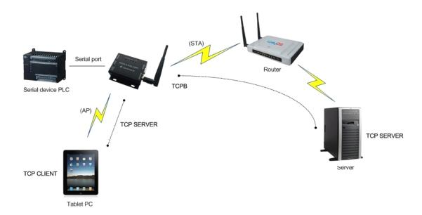
In the picture, USR-WIFI232-62E use the AP+STA function, module STA interface can be connected to router, and network server through TCP connection. At the same time, the module AP interface is also available, cellphone/PAD ect can connect to AP interface(through TCPB connection) to control serial equipment or set the module.
