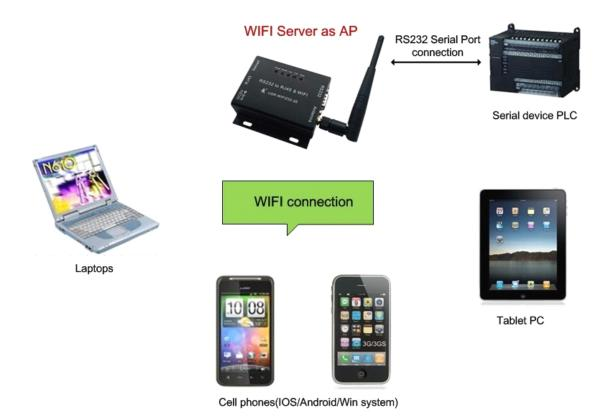
As shown in Figure, USR-WIFI232-62E used as AP. Other modules and computers can be used as a STA to connect to this module. Also, it can connect to users equipment through UART or GPIO.
