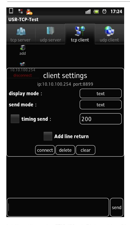
Android network test assistant(TCPIP UDP test). This is a tool that cellphone or tablet debugging for TCPIP, Configure WIFI to serial port mode, it can realize the cellphone debugging serial communication.
