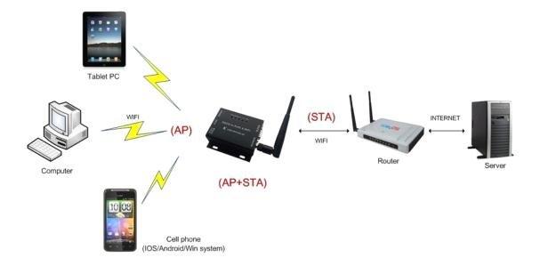
USR-WIFI232-62E can support AP+STA mode. That is the module support a AP interface and a STA interface at the same time.
