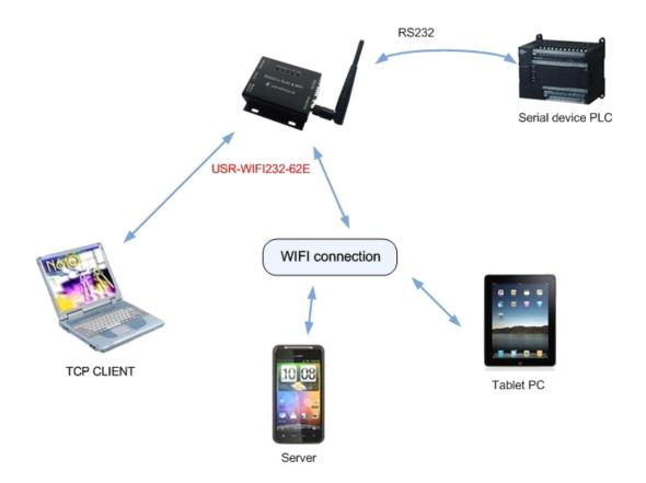
USR-WIFI232-62E support serial to Ethernet and serial to WIFI communication at the same time. As shown in picture, USR-WIFI232-62E set as TCP Server, support Ethernet and WIFI communicate with module at the same time. If module as TCP Client, serial port will access to TCP Server to communicate automatically.
