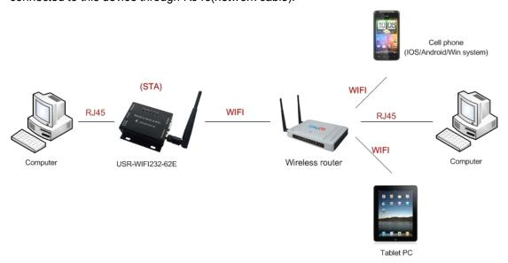
When USR-WIFI232-62E used as STA, network port connected to computer via RJ45, wireless added to wireless router to networking.
