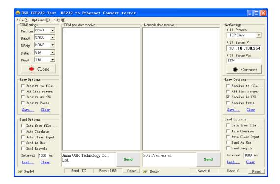
USR-TCP232-Test.exe is developed by Jinan USR IOT Technology Co., Ltd, the serial port and network commissioning test software combo.
