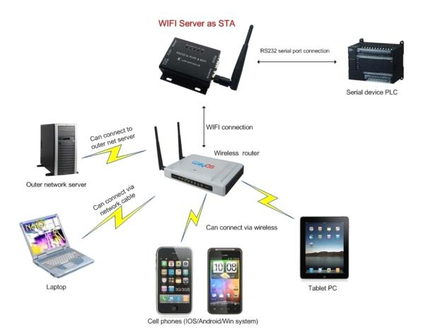
USR-WIFI232-62E as STA(use the AP CLI interface), connect to other AP, to compose a wireless network. All of the STA take AP as the wireless network center, and the mutual communication between STA is through AP forwarding.
