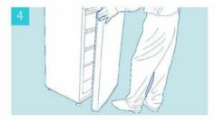
Remove the lower door from the bottom hinge pin. Tilt the fridge backwards and rest it on a firm surface.
