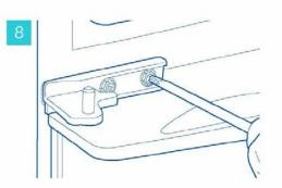
Replace the central hinge while refitting the lower door, To assist with final adjustment do not fully tighten the hinge screws.
