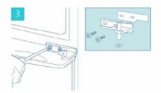
While supporting the lower door, remove the central hinge by removing the 2 screws..
