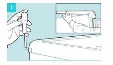
Undo the four retaining screws on the rear of the worktop and remove the worktop
