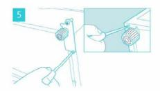
Remove the bottom hinge by removing the screws. Swap the adjustable foot from left side to right side removing the fixed screw in the left side first.
