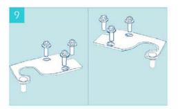
Unscrew the hinge pin from the top hinge using the spanner. Turn the hinge over and replace it in the same slot. (Reversed)
