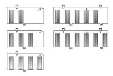
The PCI expansion bus is a field-installable backplane that you need when you configure an open controller system with any of the available option modules. You install the PCI bus in a series B 1746 chassis. You only need one PCI expansion bus per open controller chassis.
