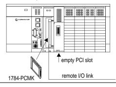
If you use a 1747-OCPM1 module with a 1784-PCMK card, use the dual port API to configure and control local I/O.
