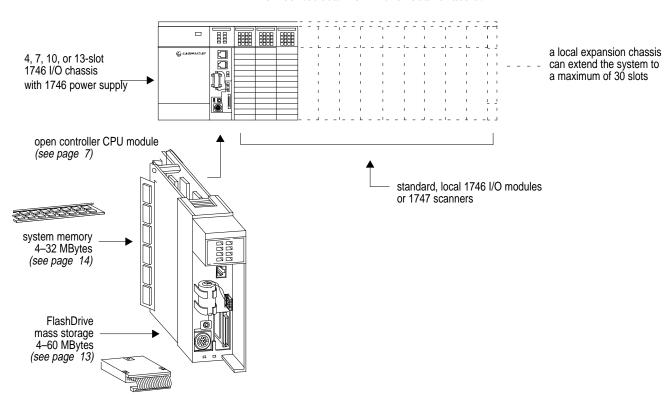
This configuration could be appropriate where only a control algorithm is needed with no typical, PC-like requirements (such as video) or network communications (such as Ethernet).
