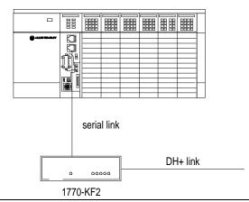
If you use a serial communication bridge, you must either write your own serial driver or use a commercially-available driver that offers the features you need. The 1770-KF2 serial bridge provides a user manual that explains how to send commands over a serial link to the 1770-KF2 bridge to communicate with devices on a DH+ network.
