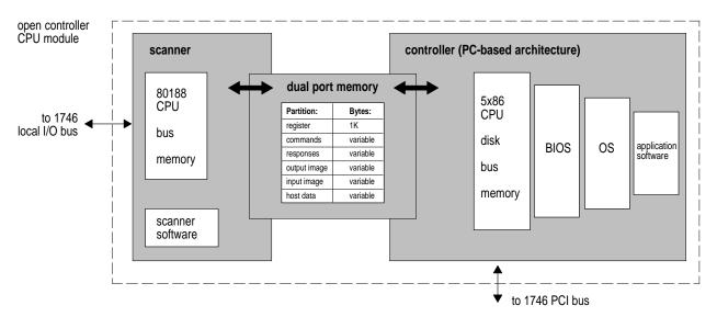
The dual port is an 8K byte memory partition that provides an interface between the integrated scanner and your application software that resides on the controller.
