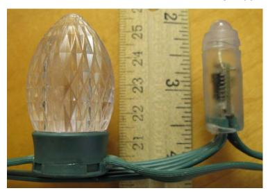
There are 50 integrated circuits (ICs,) one in each bulb. Each of these ICs can be controlled independently. The IC provides 256 levels of brightness for red, 256 levels for green and 256 levels for blue, allowing for 16 million colors.
