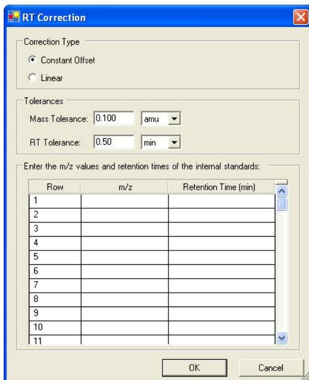
The following items control how retention time correction is performed:
