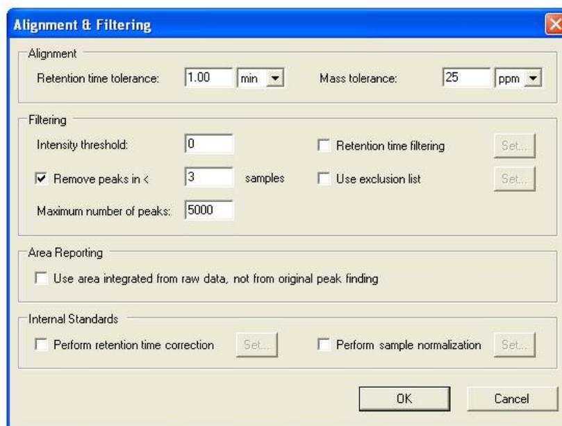
The alignment parameters are used to decide if two {mass, RT} peaks found in two samples represent the same underlying chemical component or not. If their retention times and masses are both within the specified
