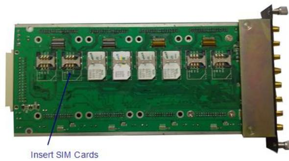
Figure 2-2-3 Push in the GSM user board
