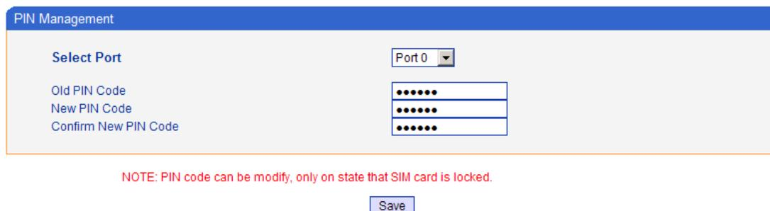
NOTE: PIN code can be modify, only on state that SIM card is locked.
