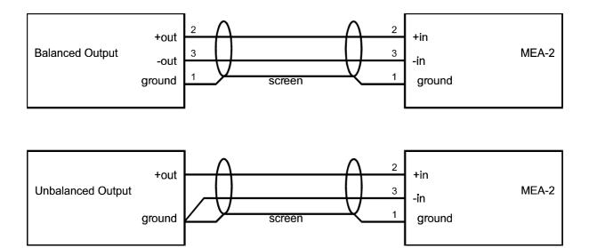
Using the above method when driving the MEA-2 with unbalanced sources should provide best results.
