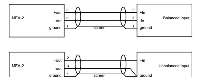
Using the above method for driving unbalanced loads should provide best results. It employs 'Ground Loop Compensation' and the signal level remains unchanged compared to balanced operation.
