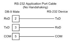
**Note:** For most null modem connections where hardware handshaking is not required, the *Use CTS Line* parameter should be set to **N** and no jumper will be required between Pins 7 (RTS) and 8 (CTS) on the connector. If the port is configured with the *Use CTS Line* set to **Y**, then a jumper is required between the RTS and the CTS lines on the port connection.
