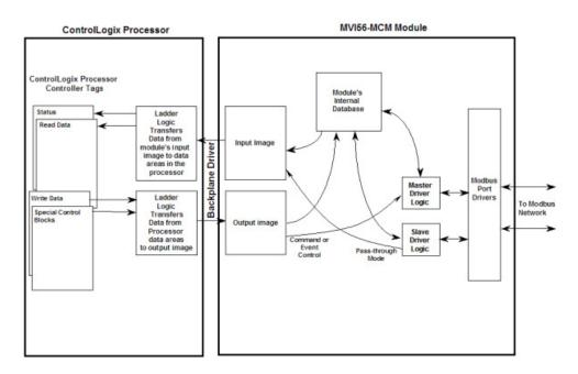
As shown in the illustration above, all data transferred between the module and the processor over the backplane is through the input and output images. Ladder logic must be written in the ControlLogix processor to interface the input and output image data with data defined in the Controller Tags. All data used by the module is stored in its internal database. This database is defined as a virtual Modbus data table with addresses from 0 to 6999.
