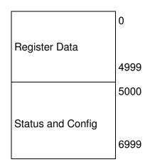
Data contained in this database is paged through the input and output images by coordination of the ControlLogix ladder logic and the MVI56E-MCM module's program. Up to 248 words of data can be transferred from the module to the processor at a time. Up to 247 words of data can be transferred from the processor to the module. Each image has a defined structure depending on the data content and the function of the data transfer as defined below.
