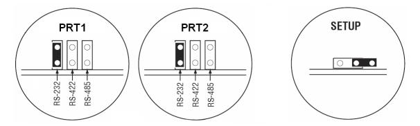
The Setup Jumper acts as "write protection" for the module's firmware. In "write protected" mode, the Setup pins are not connected, and the module's firmware cannot be overwritten. The module is shipped with the Setup jumper OFF. If you need to update the firmware, apply the Setup jumper to both pins.
