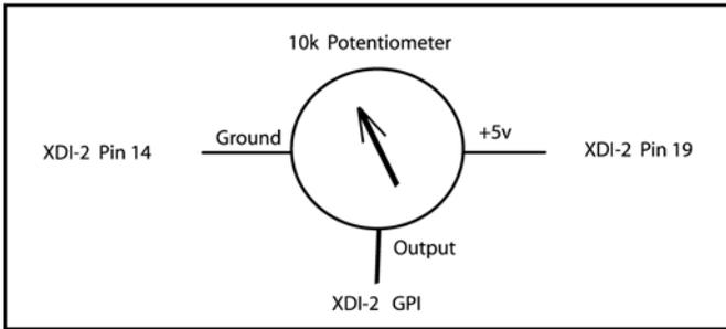
**Figure 16 :** Potentiometer wiring for Ignition and GPO Trim Inputs
