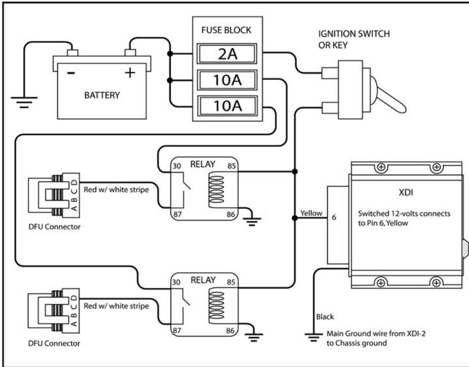
Figure 9 - Recommended power connections for a two DFU configuration
