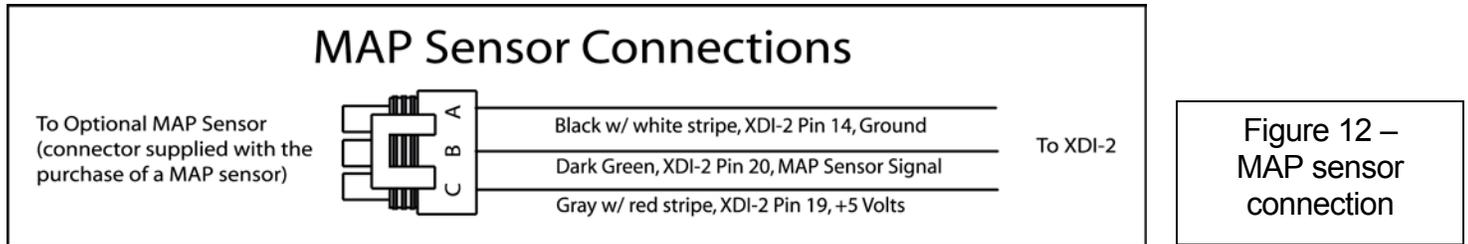
At idle, vacuum is high (manifold pressure is low), and the engine wants more advance since cylinder pressures are low. At wide-open throttle, vacuum is low (manifold pressure is high) and any additional timing is typically less than what is seen at low manifold pressure.
