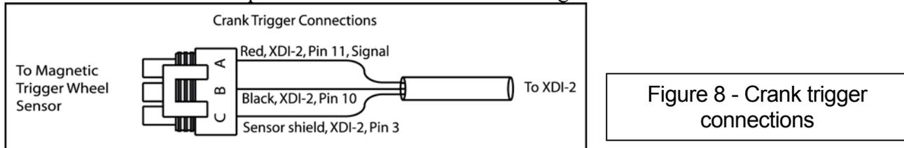
**Figure 8** - Crank trigger connections
