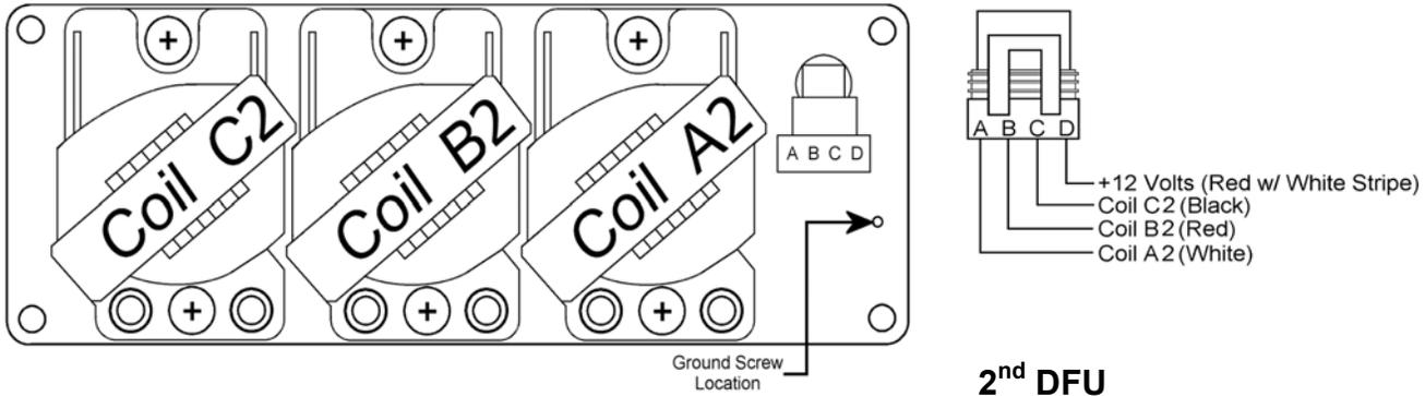
**Figure 7** - 12-Cyl, Dual Plug 6-cyl DFU setup. When used on these applications, the first DFU will have coils A1, B1, and C1, and the second DFU will have coils A2, B2, and C2.
