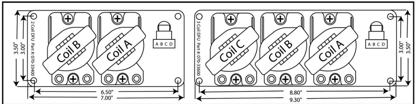
Figure 1 : 2-Coil DFU Dimensions and 3-Coil DFU Dimensions
