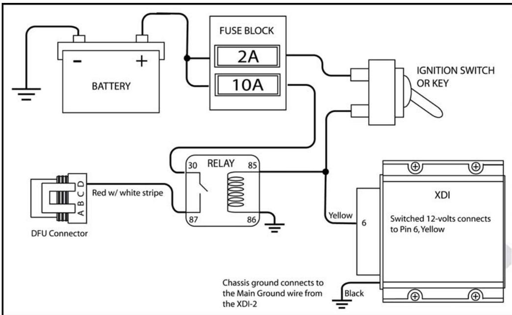
Figure 10 - Recommended power connections for a one DFU configuration
