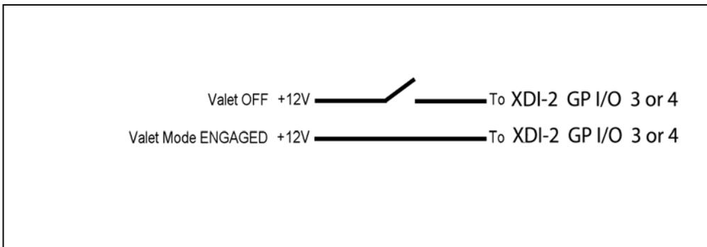
**Figure 18 :** Valet mode on/off wiring.
