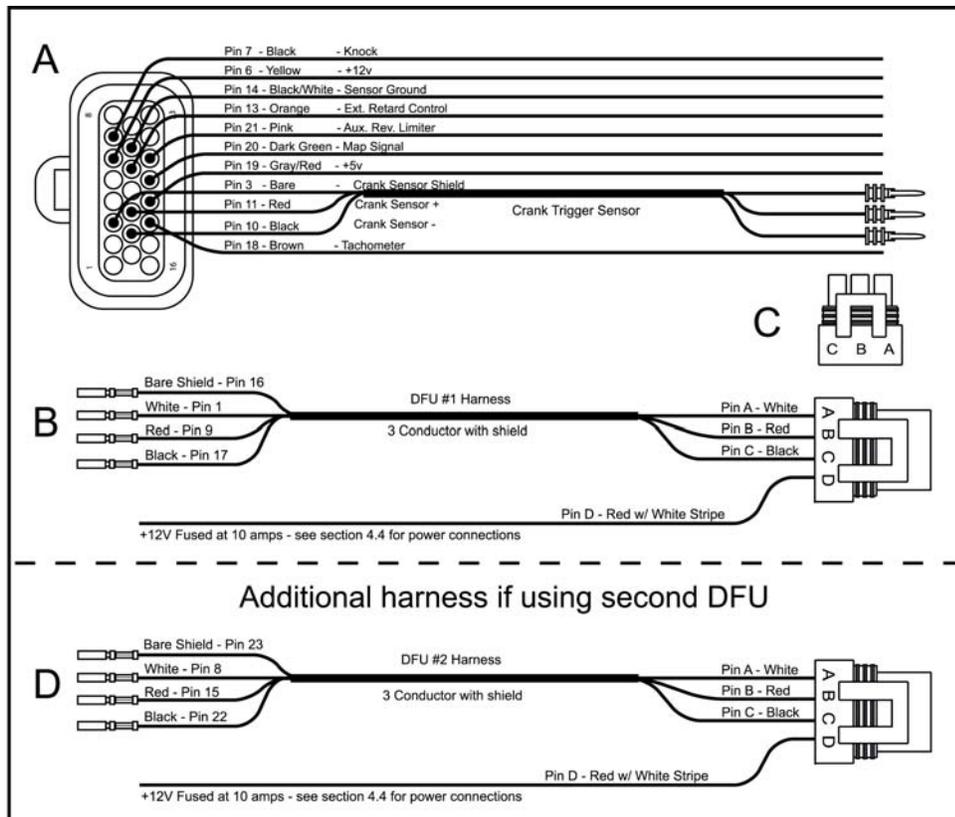
Figure 5 - Included components for wiring harness
