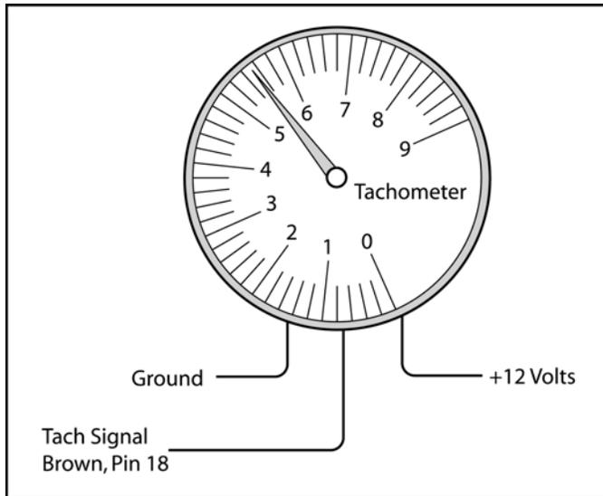
Figure 15 - Typical tachometer connections
