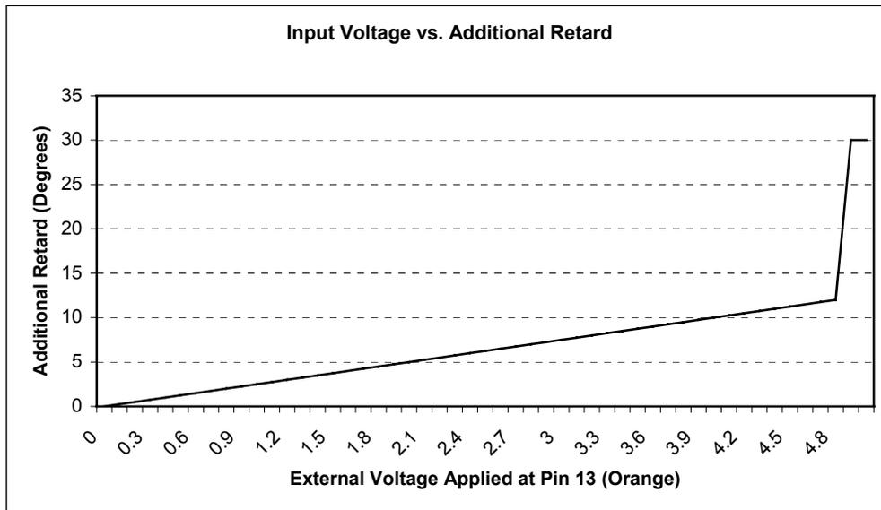
Figure 13 - Graph of input voltage vs. additional retard
