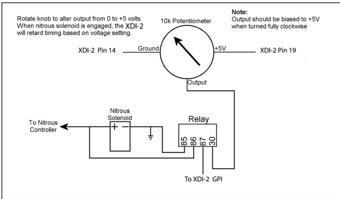
**Figure 17 :** Nitrous timing retard wiring.
