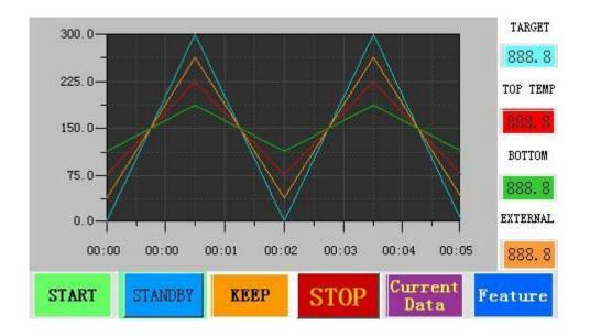
And then will appear top target temperature, top actual temperate, bottom actual temperature, actual thermostatic temperature of the third THERMATIC (preheating temperature at bottom), outer actual temperature from up to down at the right side of the touch screen.
