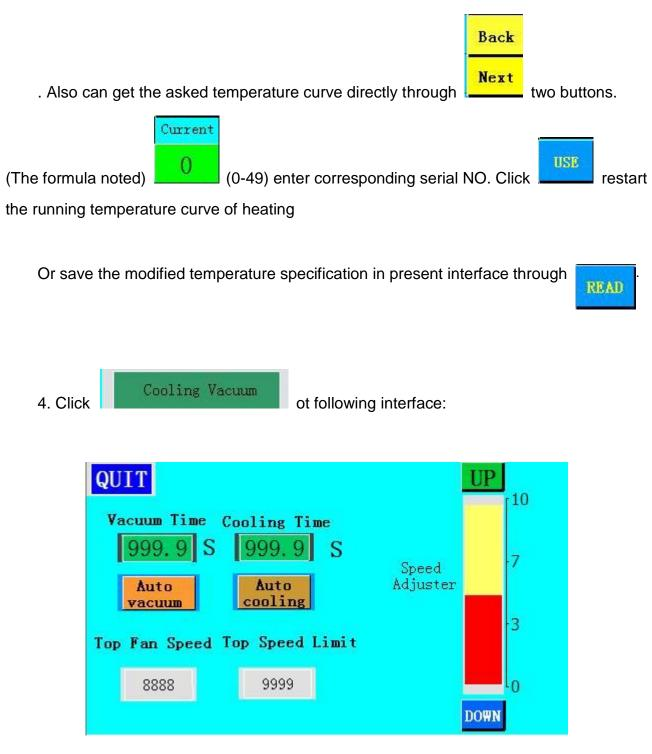
Heating finished, System will run cooling and vacuum as
