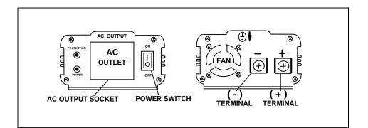
CAUTION : DO NOT REVERSE INPUT. USE RED BATTERY CORD TO CONNECT (+) OF A DC BATTERY TO (+) TERMINAL. AND THEN, USE BLACK BATTERY CORD TO CONNECT (-) BATTERY TO (-) TERMINAL.
