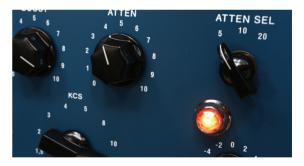
These filters are actually bit apart in frequency even if they are controlled by the same frequency selector. The High Frequency section has a peak and shelving filter working in parallel, which provides a smooth top end while not getting too bright.
