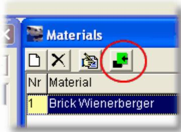
Since the only material layer in the grid is already selected, the user can simply execute the **Assign material** command and the material will be assigned to the grid. The user can now also see an assignment entry in the assignment view.
