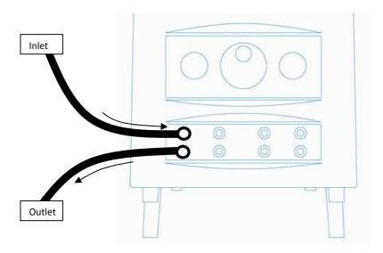
Ensure the flow direction is as per diagram above. The flow inlet is the top connection whilst the flow outlet is positioned below the inlet for each channel.
