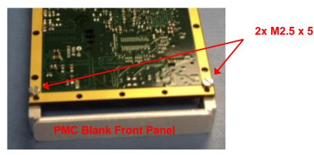
Step 2: Install the PMC/XMC module into the VPX4810 carrier by carefully angling the board so that the front panel slips though the gap in the metalwork. Once set align the connectors and gently push down until the connectors are fully inserted.
