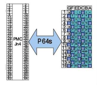
Rear I/O pin mapping diagram as defined in VITA 46.9. This product is complaint to rear I/O routing P2w1-P64s.
