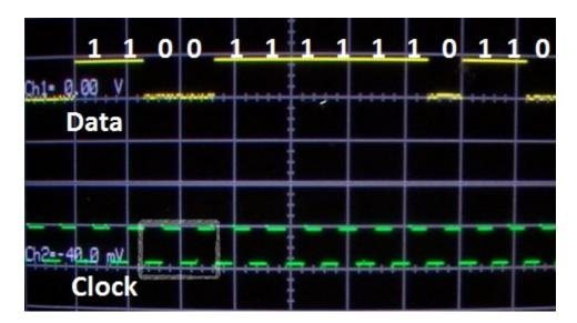
Using this mode, I could manually decode transmissions and try and determine what the data being sent looked like.
