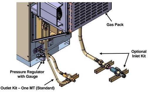
Figure 5. Single MT Installation Showing Gas Pack and Fuel Trains
