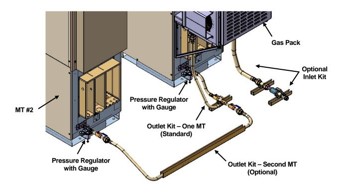
Figure 6. Dual MT Installation Showing Gas Pack and Fuel Trains
