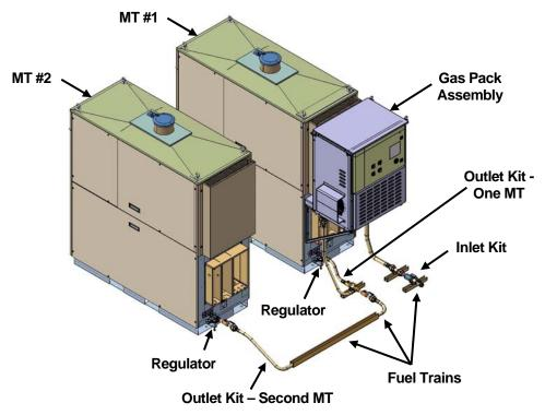
Figure 3. Installation Overview of 2 MicroTurbines, Gas Pack & Fuel Trains
