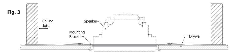
5. After the ceiling trim work is installed and the painting is complete, but just before the carpet or flooring is installed install the speaker by first connecting the speaker wire to the spring posts on the back of the speaker assembly, making sure to observe correct polarity – red (+), black (-).
