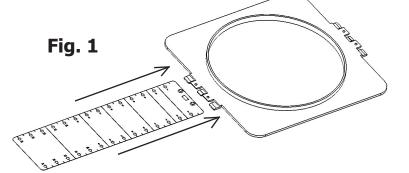
2. The wings feature progressively scored sections (1", 1", 2", 2", 2", 3", 3") with screw holes spaced in one-inch increments to help you align the bracket. The iCB6 pre-construction bracket has NHT logos on one side - this side should be oriented away from the dry-wall – towards the sky. Attach the wings to the joists using the 50mm flathead screws, use two screws for each wing. Cut off the extra portion of the wing. (fig.2).
