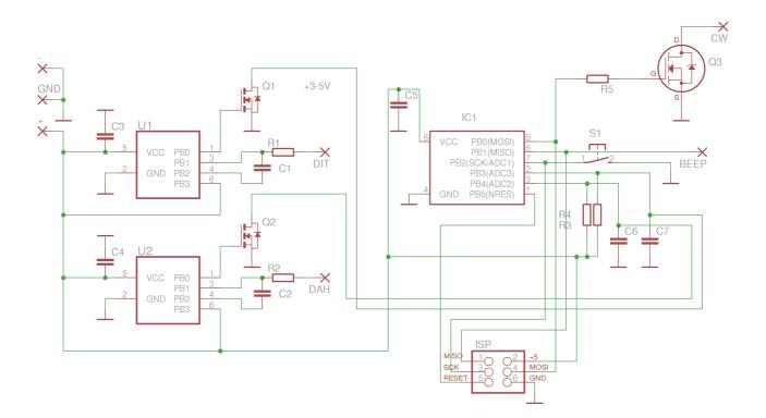
Part list: R1, R2 - 10k R3, R4,R5 - 1k C1,C2 - 2n2 C3,C4,C5 - 100nF C6, C7- 10nF U1,U2 - AT42QT1011 Q1,Q2,Q3 - IRFML8244TRPbF
