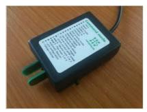
At first populate board with all SMD parts. Be careful with soldering of switch S1. The pins of switch S1 need to be cut to same level as botton of the board. The holder of S1 is soldered from the top side only. See pictures. To the box drill hole with 5 mm diameter for S1. For dimensions see picture. The on/off swith is mounted to the top side of the box. See picture for details.
