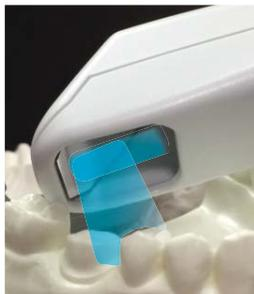
**Distal Tip** - Rest the end of the scanner tip on the distal neighbor; rock the scanner to point the blue laser into the mesial interproximal area.
