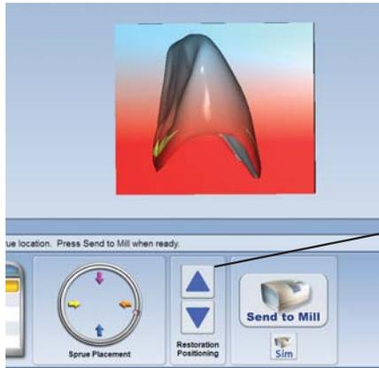
Use **Restoration Positioning** to move the proposal up or down within the block.
