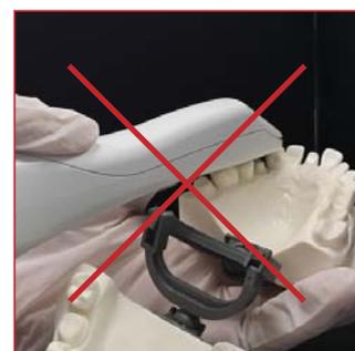
The tip of the scanner must point toward the distal of the preparation. If you scan in the incorrect orientation, you will need to delete those scans and start over.
