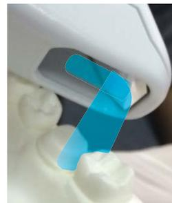
**Mesial Tip** - Rest the neck of the scanner tip on the mesial neighbor, rock the scanner to point the blue laser into the distal interproximal area.
