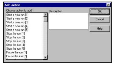
This window allows you to select the action you want the Squirrel to perform. You can define up to five instances of each action, each triggered by a different equation specifying the set of conditions that will cause the event. An identifier number is shown in parentheses after the action description.
