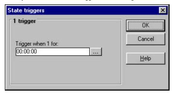
In this you can set the period for which the state trigger must be in the chosen state, before the trigger will fire. The state that will make the trigger fire is fixed when you select the trigger as it is added.
