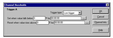
In this window you can set the threshold below which the trigger condition is met, and the length of time for which the condition must last before the trigger is fired. You can set the time by clicking the button at the right-hand end of the time field to display the **Trigger start** window:
