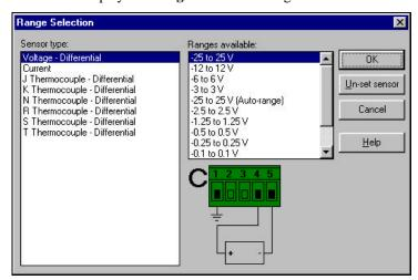
Click an option in the **Sensor type** list, and the ranges available for that sensor will be displayed in the **Ranges** available list. The range selection determines the resolution of the readings as well as the maximum and minimum values that can be logged. You can select the appropriate range then click the **OK** button to apply the selections.
