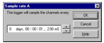
To change a setting in any time field, click the field then use the arrow buttons to adjust to the required value.
