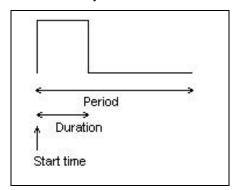
As most actions are edge-trigged (they only notice transitions from false to true and vice versa) the value set for the duration will not be needed; however, you will still need to enter a duration with a value less than the trigger period.
