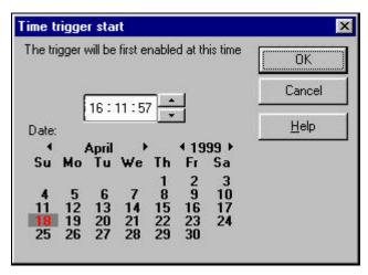
To change a setting in any time field, click the field then use the arrow buttons to adjust to the required value. You can change the month and year using the arrows adjacent to their labels, then choose a different date either by clicking the required date or using the **ARROW** keys on your computer keyboard.
