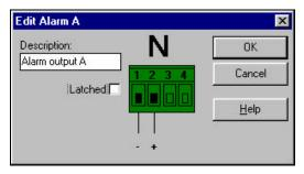
You can enter a description that will be used to identify this alarm type, up to 20 alphanumeric characters. You can also set the alarm to be latched (causing the alarm to continue until it is reset through either the Status tab or the Squirrel control panel) or unlatched (causing the alarm to be reset as soon as the alarm condition is removed) by selecting or deselecting the **Latched** checkbox. Alarm conditions are determined by equations defined in the **Actions** tab.
