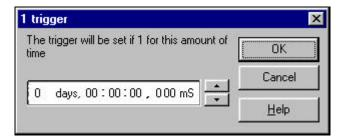
To change a setting in any time field, click the field then use the arrow buttons to adjust to the required value.
