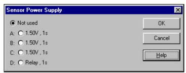
The options available in this dialog box represent the power supplies set up in the **Logger** tab. You can choose the option button corresponding to the required power supply then click the **OK** button.
