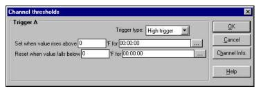
In this window you can set the threshold above which the trigger condition is met, and the length of time for which the condition must last before the trigger is fired. You can set the time by clicking the button at the right-hand end of the time field to display the **Trigger start** window:
