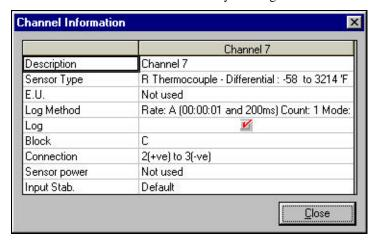
Note that entries and changes made in this window will be lost when the window is closed. If you want to change the channel details, select the **Analogue** tab and use the procedure described in **Analogue channel settings**.
