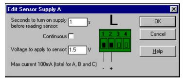
You can enter the number of seconds for which the supply will be switched on before a reading is taken, or select the **Continuous** checkbox to have the supply on all the time. You can also enter the output voltage supply, in increments of 0.05 V.
