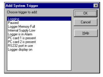
In this window you can select the required trigger then click **OK**. This will display an **Edit** window in which you can edit the operating parameters for the trigger. The content of this **Edit** window will depend on the type of trigger selected.
