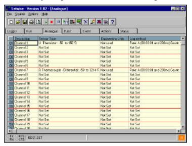
Note that temperature sensor values are converted from either resistance (for thermistors) or voltage (for thermocouples) into degrees Centigrade or Fahrenheit.
