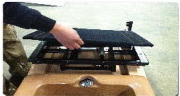
After removing the bolts, flip the black cover support up
