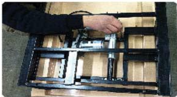
Install four bolts and washers to secure the metal frame to the base tub
