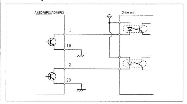
Fig. 2 Example of connection to A1SD75P□/AD75P□ open collector
