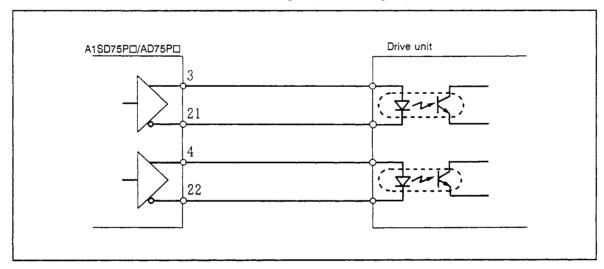
Fig. 1 Example of connection to A1SD75P□/AD75P□ differential driver
