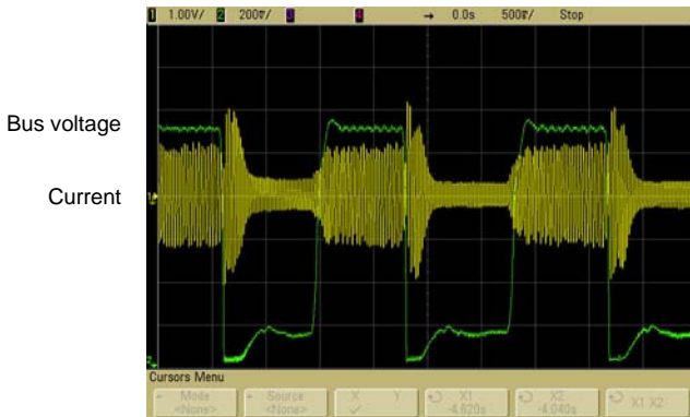
Fig. 2 The Asynchronous servo drive realizes stable control of current and voltage and will not trigger under any acceleration/deceleration condition as well as stable operation condition
