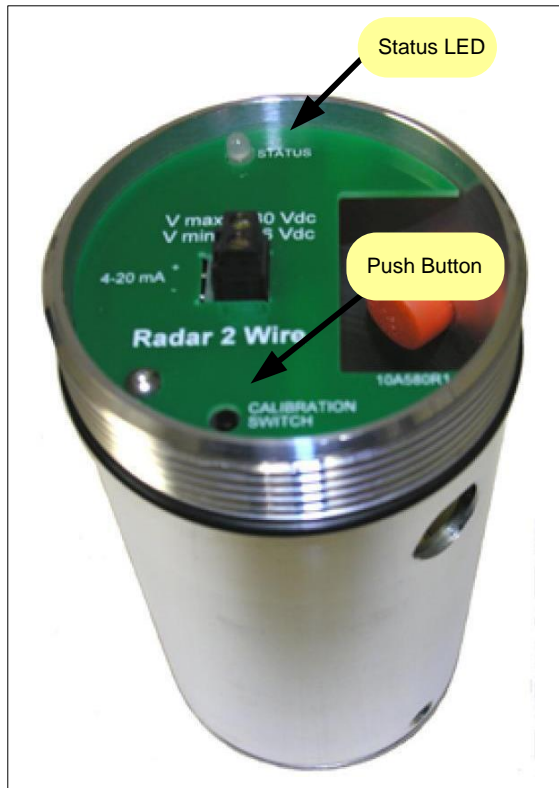
Figure 27. The illustration shows the location of the LED and the push button for both Radar and Ultrasonic sensors.
