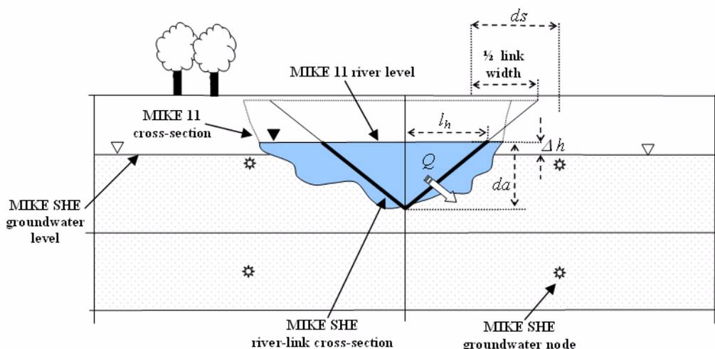
Figure 7.11 A typical simplified MIKE SHE river link cross-section compared to the equivalent MIKE 11 cross-section.
