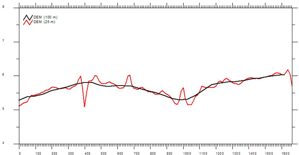
Figure 7.9 Example of preprocessed data - topography using a 100 meter resolution and a sub-scale factor of 4 (25 m sub-scale resolution).
