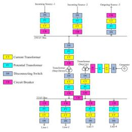
Figure 2: Block diagram of a primary substation
