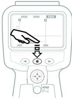
Backlight key. Press the backlight key to switch the backlight on. It will switch off after one minute with no key press when activated, or it may be switched off by pressing the key again
