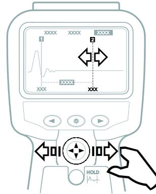
Moving the four-way switch left or right will move the active cursor.
