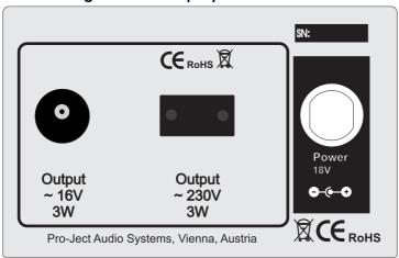
Turntables without an external AC power supply should be connected to the **Output** socket (50Hz models to **Output ~230V 3W** / 60Hz models to **Output ~120V 3W**) on the Speed Box DS. Check the label before connecting to ensure compliance with the mains rating in your house.
