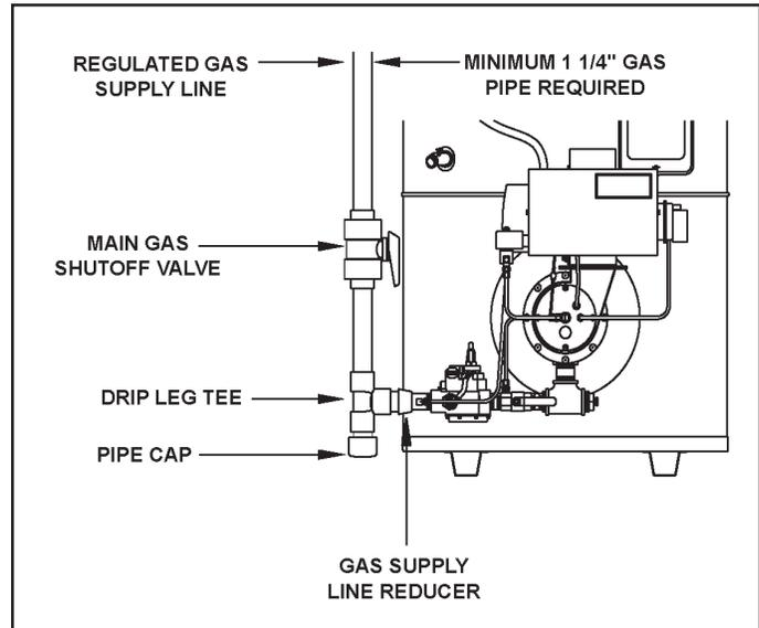
**GAS PIPING AND DIRT LEG INSTALLATION**
