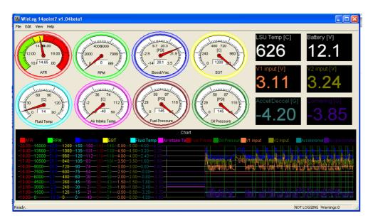
If SLC DIY 2 is connected to your PC via USB and the Comport# is correctly set, the dashboard should be updating with live data from SLC DIY 2.
